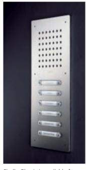
Siedle Classic is available for flush-mount installation in a width of 170 millimetres as standard. In the standard version, the audio door station accommodates a maximum of eight keys, the video model a maximum of four. Special versions can be produced with the dimensions enlarged in fixed grid steps to accommodate additional keys or to achieve different measurements.
