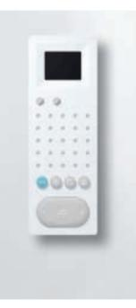
The large call button, the door opener, light switch and mute key are common to both audio and video devices. The fourth key of the video model switches the door camera manually to the monitor, with the camera picture being displayed automatically each time the door rings. Two control knobs for colour saturation and brightness adjust the reproduction on the 2.5-inch colour screen.
